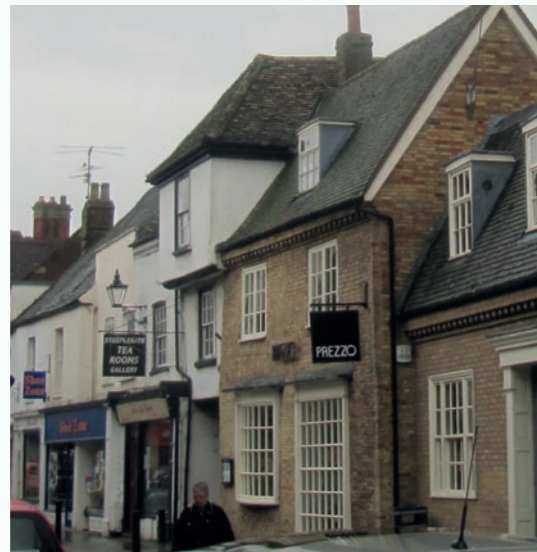
Figure 4.36: Informal buildings on the edge of Ely Town Centre have varied window proportions that make the building group appear complex. This complexity is 'calmed down' by the consistency of degree of roof pitch pitched roofs and building line
